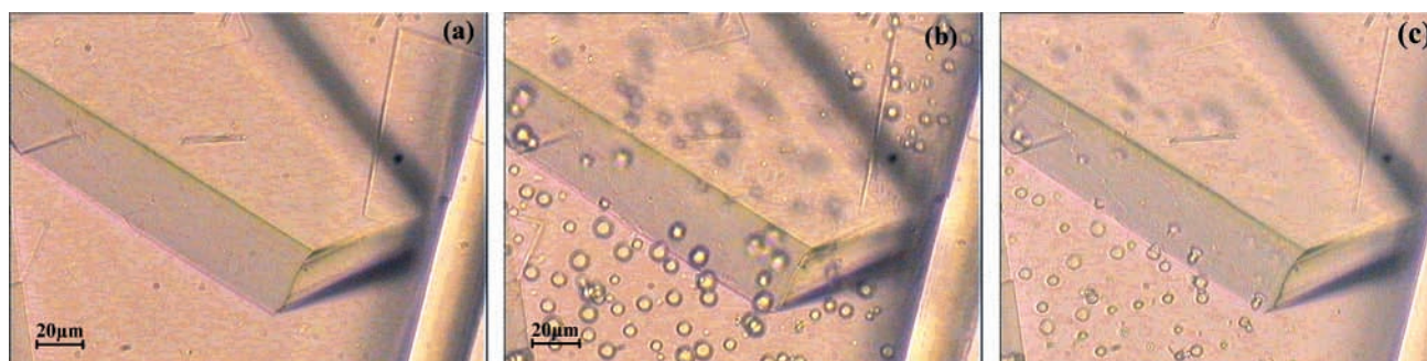
Figure 3. Observation by optical microscopy of the nucleation of droplets of the protein-rich phase in a supersaturated solution of BPTI (24 mg/mL) when the temperature is decreased: (a) T = 20\text{ }^\circ\text{C} ( \beta = 1.4 ) and (b) T = 15\text{ }^\circ\text{C} ( \beta = 2 ). And dissolution of droplets when the temperature is increased from 15 to 20 °C (c).
